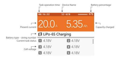
Rotating the shuttle key during operation can switch the displayed information in the lower half of the screen, which are cell voltage, cell internal resistance and working parameter. The cell voltage and internal resistance can only be displayed in the mode of balance charging.
